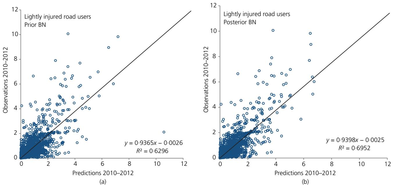
Figure 5. Comparison of predicted against observed number of accidents with light personal injury with prior BN model (a) and with posterior BN model (b)
