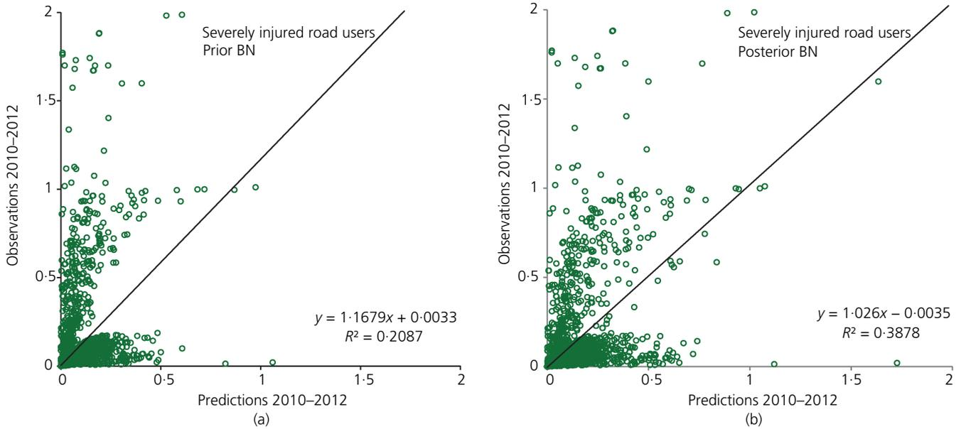
**Figure 6.** Comparison of predicted against observed number of severe and fatal injury accidents with prior BN model (a) and with posterior BN model (b)
